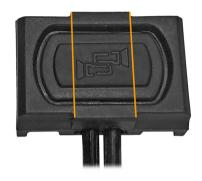
DETERMINE WHICH GENERATION THE MODBUTTON LITE IS. OLD GENERATION REQUIRES NO MODIFICATION. NEW GENERATION CAN BE IDENTIFIED USING PAPER OR A CARD TO DRAW A LINE FROM EITHER SIDE OF THE MATING TABS. IF THE FLASHLIGHT LOGO IS FULLY VISIBLE IT IS A NEW GENERATION. NOTE: A SINGLE WIRE DOES NOT NECESSARILY MEAN THE MODBUTTON LITE IS AN OLD GENERATION.
