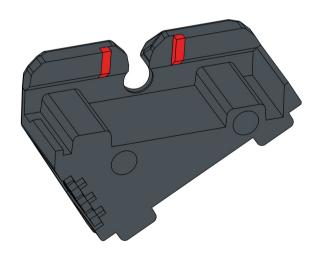
2 LOCATING THE MATING TABS ON THE RAMP OR DUAL RAMP PRODUCT AND REMOVE 0.05" (ROUGHLY THE THICKNESS OF A PENNY) OF MATERIAL FROM EACH SIDE AS SHOWN HIGHLIGHTED IN RED. DOUBLE CHECK FITMENT WITH YOUR NEW GENERATION MODBUTTON LITE TO CONFIRM THE AMOUNT OF MATERIAL REMOVED IS CORRECT. THE MODBUTTON LITE TABS SHOULD HAVE A SNUG FIT IN THE RAMP.
